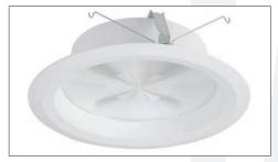
**Eaton's** Cooper Lighting PR8 by Halo was accepted as the first 8-in. diameter LED downlight to feature selectable CCT and selectable wattage/drive current dip switches. With over 120 lpw, light output options are available in 1,000 to 4,000 lumens and with a wet-location listing.
