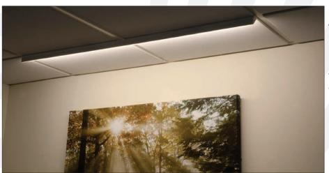
From **JLC-Tech** comes the T-BAR LED Asymmetrical family of luminaires. This unique fixture, which incorporates a proprietary multi-ribbed lens that bends light by 30 deg, mounts 1 to 2 ft from the wall replacing a piece of the grid in the ceiling system.
