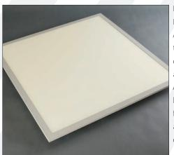
First up is the Forum LED Panel Lite from **Liteline Corporation**. At an overall depth of 1-% in. the fixture provides even light distribution across the entire panel at an efficacy of up to 125 lpw. Available in 2 by 2, 1 by 4, and 2 by 4 configurations, this is the first field-selectable color temperature and wattage panel with no external controls needed.
