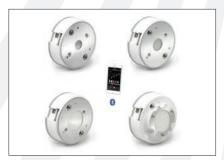
LED Dual Profile araya5 Tuning Module from **Lumenetix** is the first LED module featuring the combination of dynamic color tuning, dimming and Bluetooth connectivity. It mixes five colors, and features two user-selectable lighting profiles of Dynamic Dimming and Tunable Color. The former matches halogen intensity and CCT shift, and the latter independently tunes intensity, CCT from 1650K to 8000K, color hue and saturation.
