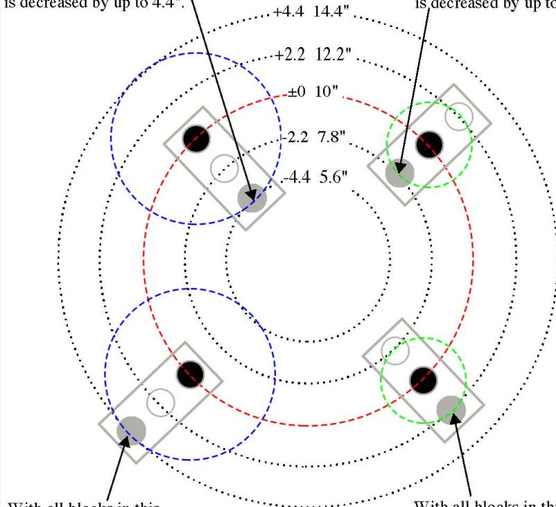
With all blocks in this configuration, the bolt circle is increased by up to 4.4".
